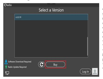
Obtaining a SmartSDR software license using an M model FLEX-6000 or a Maestro is easy and convenient. After downloading and installing a SmartSDR 3 software version, At the Select a Version screen, choose the version 3 software just installed. If you need to purchase a license to run the software, the Buy button will appear as shown below.
