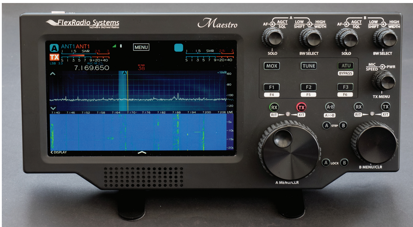
The Maestro is a standalone unit that enables full control of any FLEX-6000 series of transceivers.
