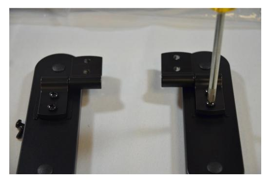
Prepare Hinge-Foot Assembly for Attachment to Maestro
