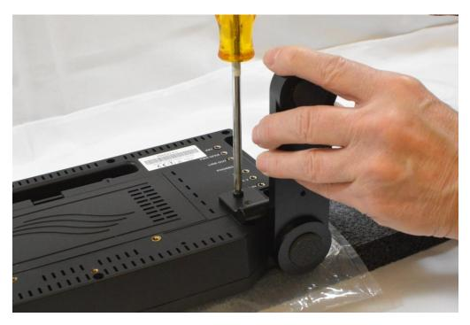
Below shows an image of the completed installation of both hinge-foot assemblies.
