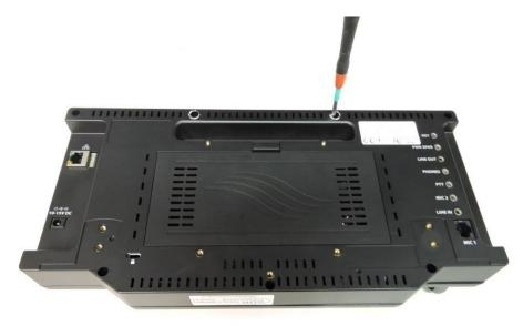
Using the #2 Phillips screwdriver, reinstall the tilt feet or the fixed tilt stand on the Maestro.
