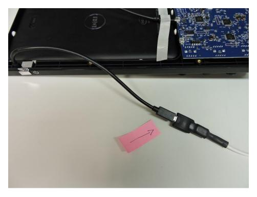
In the Charging cable, connect the USB A (male) connector to the low amperage USB charger. The charger can be powered by a laptop's USB port or a Smartphone battery charger that accepts a USB A cable. Allow the Internal Display battery to charge for **at least one (1) hour**. Do not use a high amperage tablet charger as the display requires an initial "slow charge" for proper battery re-charging.
