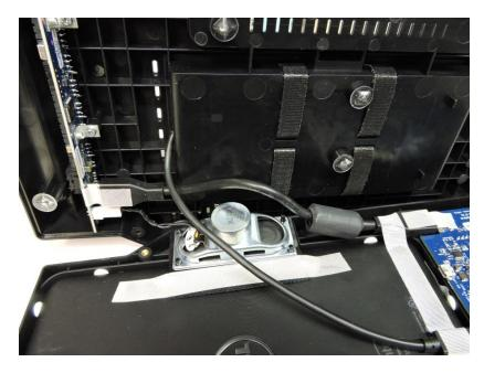
Once the cables are oriented correctly, carefully close both halves of the Maestro chassis together ensuring that none of the cables have been pinched.
