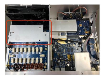
**Step 5:** Remove EXT TX with attached mounting platform from bag. Remove the EXT TX board from mounting platform by removing the three screws.
