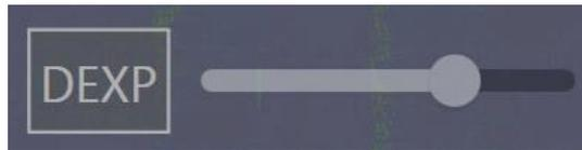
The Downward Expander controls are found in the **TX Menu**. The Downward Expander reduces the microphone input gain during the quiet periods between spoken words, eliminating extraneous background noise. This improves the apparent signal to noise ratio of your transmitted audio by “soft gating” ambient room noise between words.
