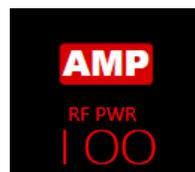
When the button is red, the amplifier is engaged and amplifying the RF signal sent by the transceiver.
