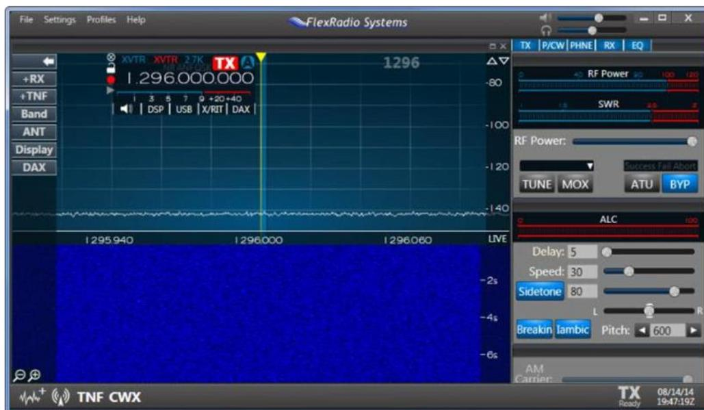
The FLEX-6000 is actually receiving on the programmed IF frequency but performing a frequency translation in the Slice and the Panadapter to indicate the frequency being listened to.
