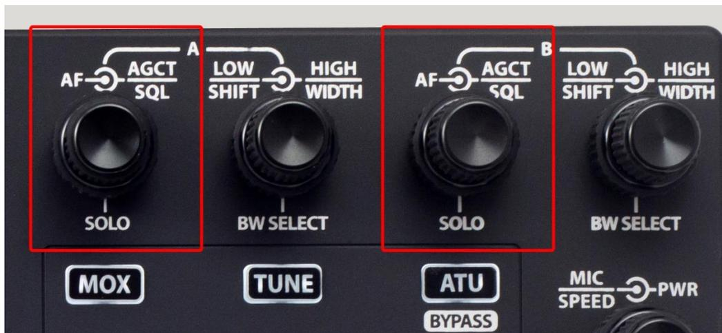
These multi-function knobs control audio level, AGC threshold and solo channel operation.
