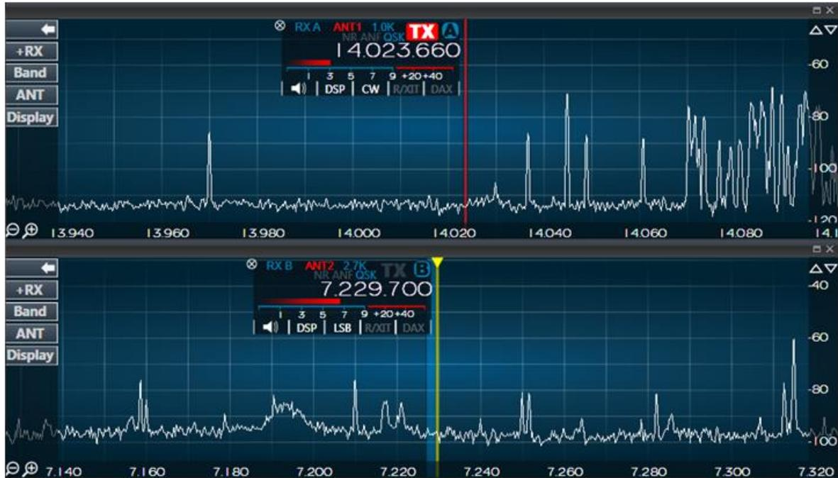
In the image above, a FLEX-6600M is configured so that the Slice A receive antenna is set to RX A and the Slice B antenna to RX B. ANT1 is selected as the transmit antenna for Slice A and ANT2 for Slice B. This configuration allows separate receive antennas on the two independent SCUs. This configuration is not available on the single SCU FLEX-6400M.
