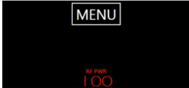
The center of the display upper bar features indicators showing the RF Power Amplifier output level and a button to open the **Main Menu**. See section 31, **Main Menu** for full details about the **Main Menu**.
