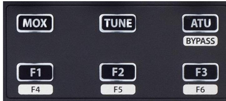
The function buttons provide a means to map a selection of radio operations to front panel buttons for convenient access. Mapping of the operations to the buttons is performed on the **Main Menu** Function Buttons tab. See section **31.4, Function F1-F6 Tab** for complete details.
