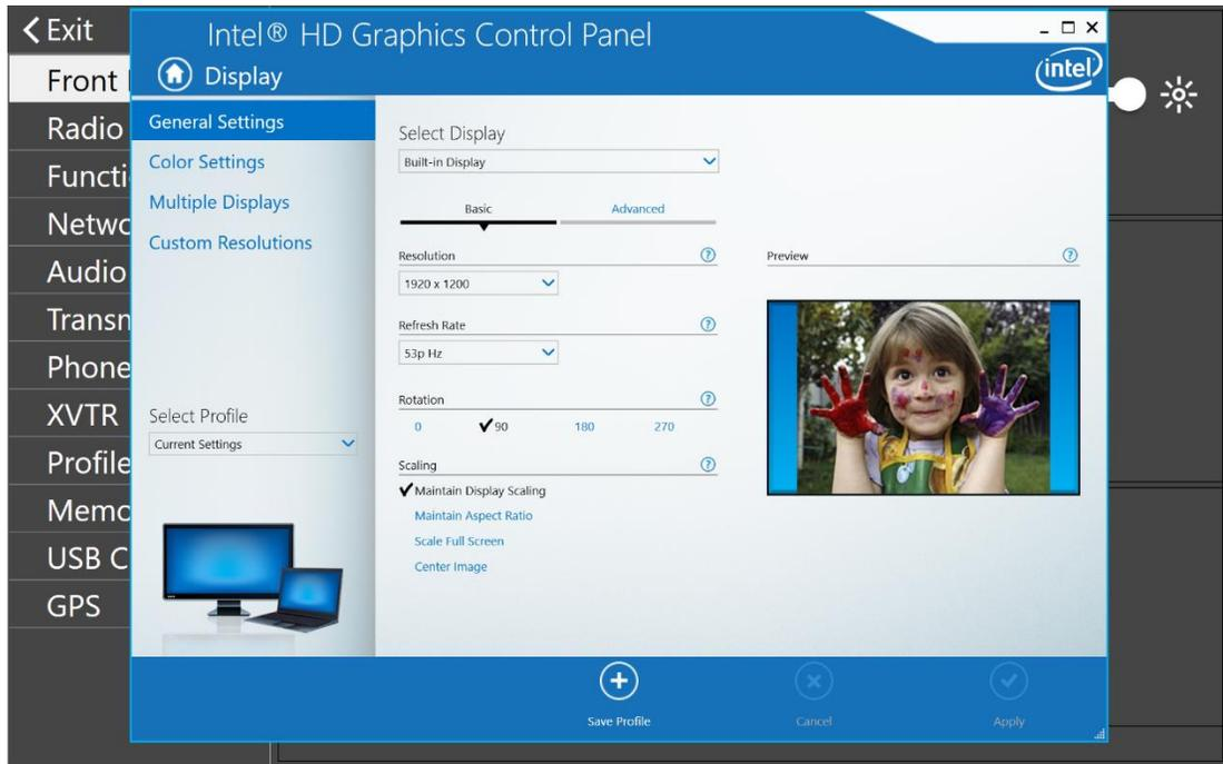
Make sure the external display is on and plugged into the back-panel HDMI port. Select the display using the drop-down menu near the top of the Display Control Panel:
