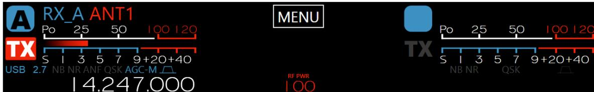
Located in the upper bar of the display are the two Slice Receiver Flags, the A Slice on the right and the B Slice on the left. In the center of the bar are the **Main Menu** button, the RF power level indicator, the power supply indicators and the network signal strength indicator. When a Power Genius XL amplifier is configured with the radio, its control appears above the RF power level.
