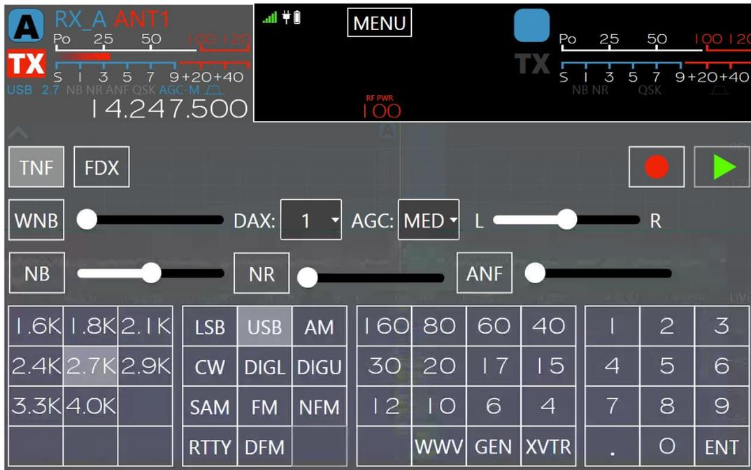
The slider to the right of the ANF button controls the depth and sensitivity of the filter. Automatic Notch Filters are not affected by the setting of the global Tracking Notch Filter control, section 15.3, **Turning all Tracking Notch Filters On or Off.**
