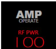
When the button reads “AMP Operate”, the amplifier is connected to the radio and ready to accept and amplify an RF signal. Tap on the button to change the amplifier state to “Standby”.
