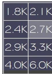
Standard SSB receive filter bandwidths from 1.6K to 6.0K can be selected from the **Slice Receiver Menu**. Custom bandwidths can be adjusted by use of the High/Low Shift/Width multi-function control. When the control is in High/Low mode, adjusting the inner knob moves the location of the lower frequency margin of the filter, while adjusting the outer knob moves the location of the higher frequency margin. Pop-up displays provide detailed information as the adjustments are made.
