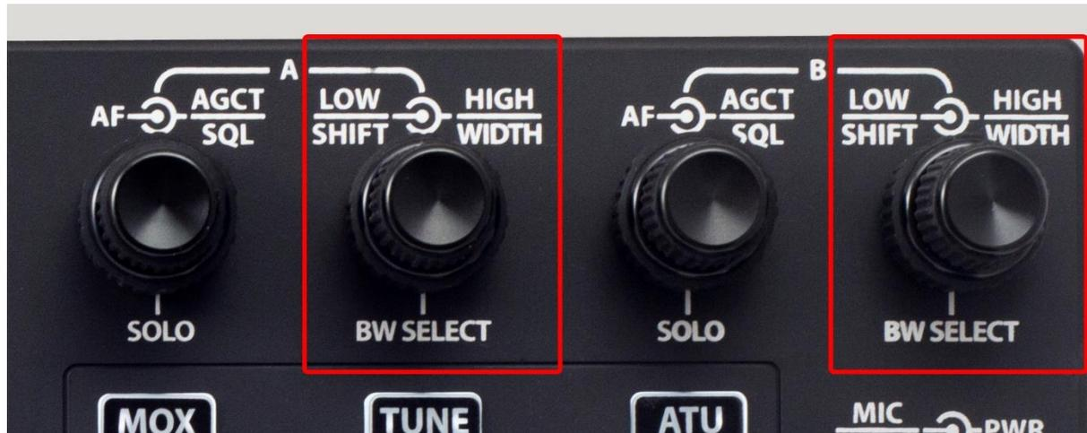
These multi-function knobs control Slice Receiver filter lower and upper bounds and the manner in which they are changed.
