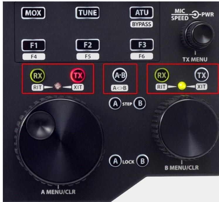
Pressing an **RX** button when the corresponding Slice is inactive causes the Slice Receiver to become active. The button will illuminate green. Pressing the button again causes the Slice Receiver to become inactive. With appropriate button presses, it is possible for zero, one or two Slice Receivers to be active.
