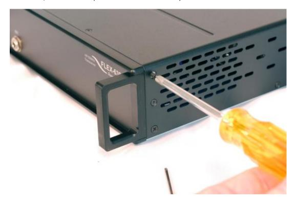
Repeat the previous procedure for installing the front side cover TORX and Phillips screws on the left side of the FLEX-6300.
