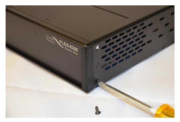
After removing both Front Side Cover Phillips screws, remove the 4-40 X ½" **Front Side Cover TORX screw** using the long portion of the "L" TORX wrench. Retain the Front Side Cover TORX screw for reinstallation. The image below shows the removal of the right side Front Side Cover TORX screw.
