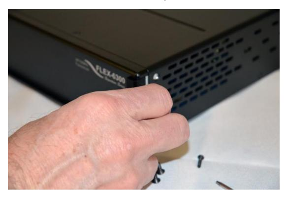
The image below shows the right Frame Bezel being removed from the FLEX-6300.
