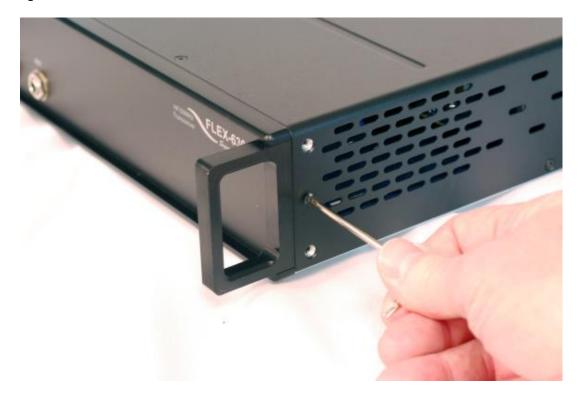
After installing the center TORX Side Cover screw, re-install both the top and bottom 6-32 x 3/8" flat head Phillips Side Cover screws using a #2 Phillips screwdriver. *Be careful not to cross-thread the screws and over tighten the Phillips Side Cover screws.* The image below shows the installation of the top Phillips Side Cover screw; the bottom Phillips Side Cover screw has already been installed.
