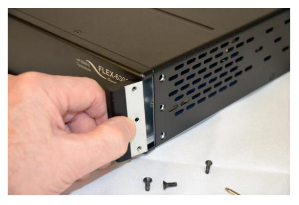
Repeat the previous procedure to remove the left Frame Bezel after the right side Frame Bezel has been removed. The image below shows both Frame Bezels removed and the radio ready for the handle installation.
