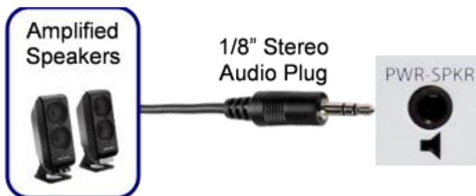
The powered speaker connector is a 1/8" TRS stereo connector. Stereo powered computer speakers should be used with this connector. The Tip is the left channel, Ring is the right channel and Sleeve is common. The audio level is a nominal standard consumer (-10 dBV) line level. Do not use a mono or TS connector that grounds the “ring” portion of the connector.
