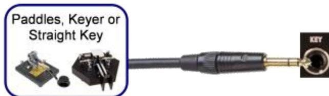
The CW key/paddle jack is a ¼ inch TRS phone plug. For an iambic paddle, the tip is connected to the dot paddle, the ring is connected to the dash paddle and the sleeve is connected to the common. For a straight key or a keyer output, connect to the tip and leave the ring floating. The common is connected to the sleeve. (Note: 3.3VC Max input.)
