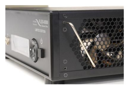
Remove the bottom **set screw** as shown below.
