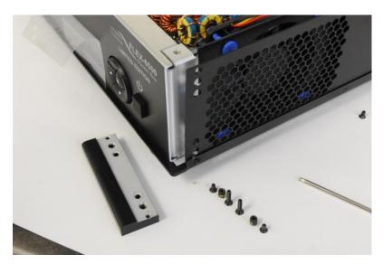
Remove the left front Frame Bezel after the right side front Frame Bezel has been removed.
