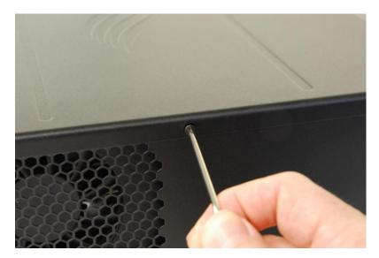
After removing the top cover side screws remove the four (4) long **Top Cover screws** using the long portion of the "L" TORX wrench. Retain the Top Cover screws for re-installation. The image below shows the removal of the Top Cover screws.
