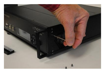
After removing the Set, Cover and Side plate screws, the corner of your FLEX-6000 should look like the image below.
