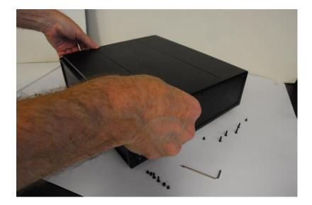
After replacing the top cover re-install the four (4) long **Top Cover screws** using the long portion of the "L" TORX wrench. *Do not over tighten the Top Cover screws.* The image below shows the removal of the Top Cover screws.
