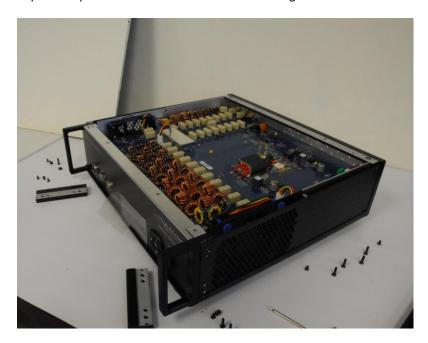
Reinstall the **Front Chassis Retaining Bar** by placing on top of the radio with the black edge facing outward and aligning the screw holes with the chassis holes. Install a chassis retaining bar screw and washer. Do not tighten the screw at this time. The image below shows the installation of right side chassis retaining bar screw.
