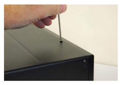
Once the top cover retaining screws have been removed, gently pull the Top Cover upwards to remove it from the FLEX-6000. The image below shows the removal of the Top Cover.
