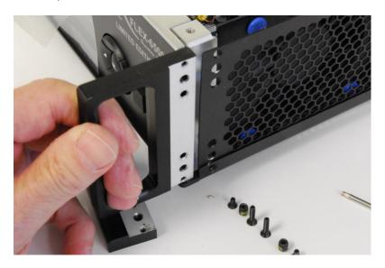
Repeat the procedure for the left handle. The image below shows both Handle Assemblies installed.
