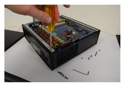
After both Front Chassis Retaining Bar screws have been removed, gently pull upward on the Front Chassis Retaining Bar to remove it from the chassis. Retain the Front Chassis Retaining Bar for reinstallation. The image below shows the Front Chassis Retaining Bar being removed.
