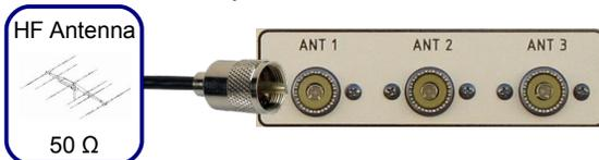
If you have the optional Antenna Tuner installed, the impedance may deviate from 50 Ohm (see the Owner's Manual)
