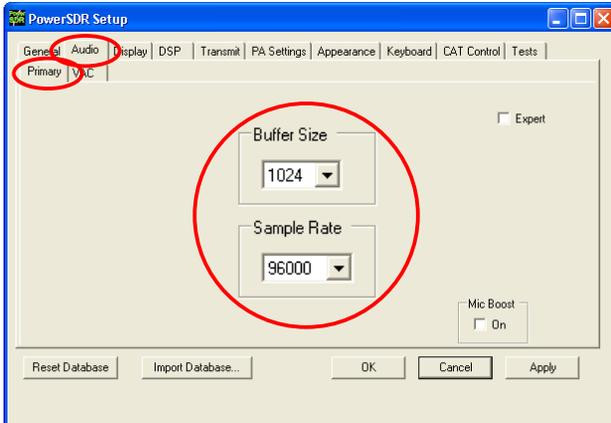
Set the **Buffer Size** to **1024** and the **Sample Rate** to **96000** (these same values have been set in the FLEX-5000 Device Driver). Click **OK** at the bottom right to complete the settings.
