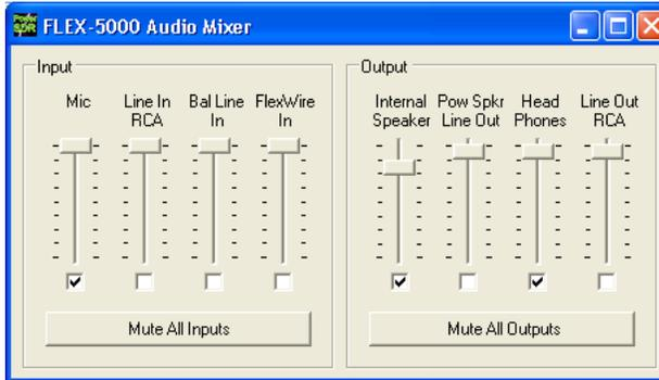
Check **Mic** as the Input to select the front **Microphone** jack. Check **Internal Speaker** as the Output, to activate your internal speaker. Check **Pow Spkr Line Out** and/or **Head Phones** if instead (or simultaneously) you want to send audio to external speakers (see Step 1-C), and/or the front **Phones** jack.
