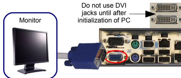
To initialize your computer you will need a monitor connected to the blue VGA jack. After initialization, you may switch to using one of the two white DVI jacks (if your monitor supports this).
