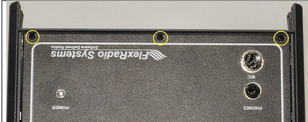
Figure 9 – Placement of the three (3) bottom screws. The other three (3) are at the top
