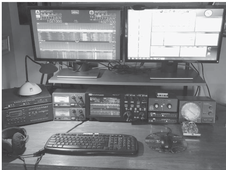
Figure 3 — KØAD's simplified SO2R contesting station with the FLEX-6600M.
